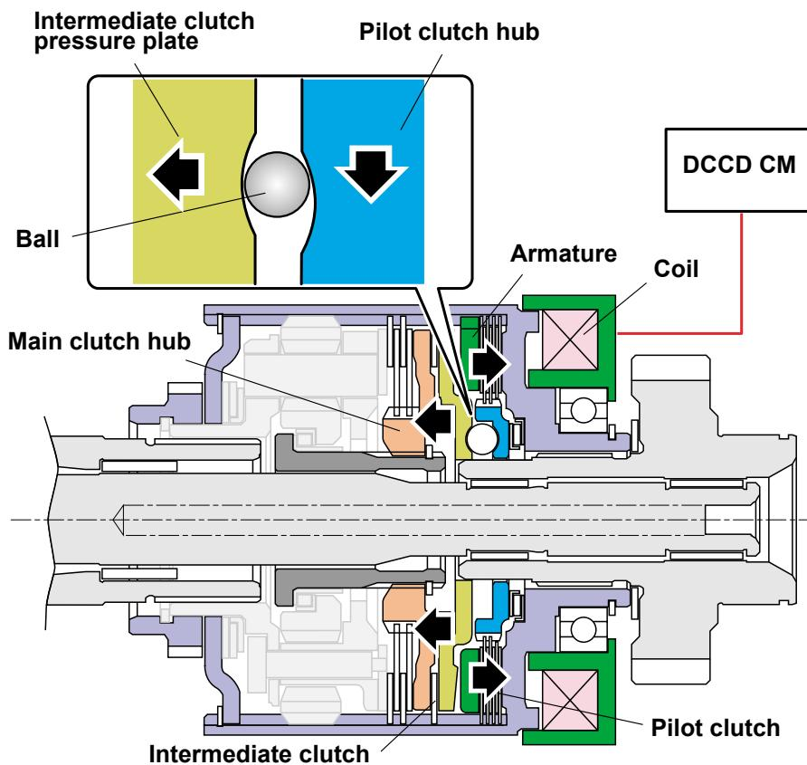
As the result, the balls placed between the intermediate pressure plate and pilot clutch hub are given a force that presses the intermediate pressure plate leftward, causing the intermediate and main clutches to be engaged with each other.
