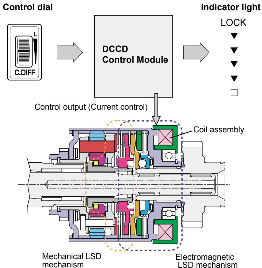
The DCCD control module gives certain current determined by setting on the control dial to the coil. It causes the magnetic clutch LSD differential limiting force to be fixed to a certain value.
