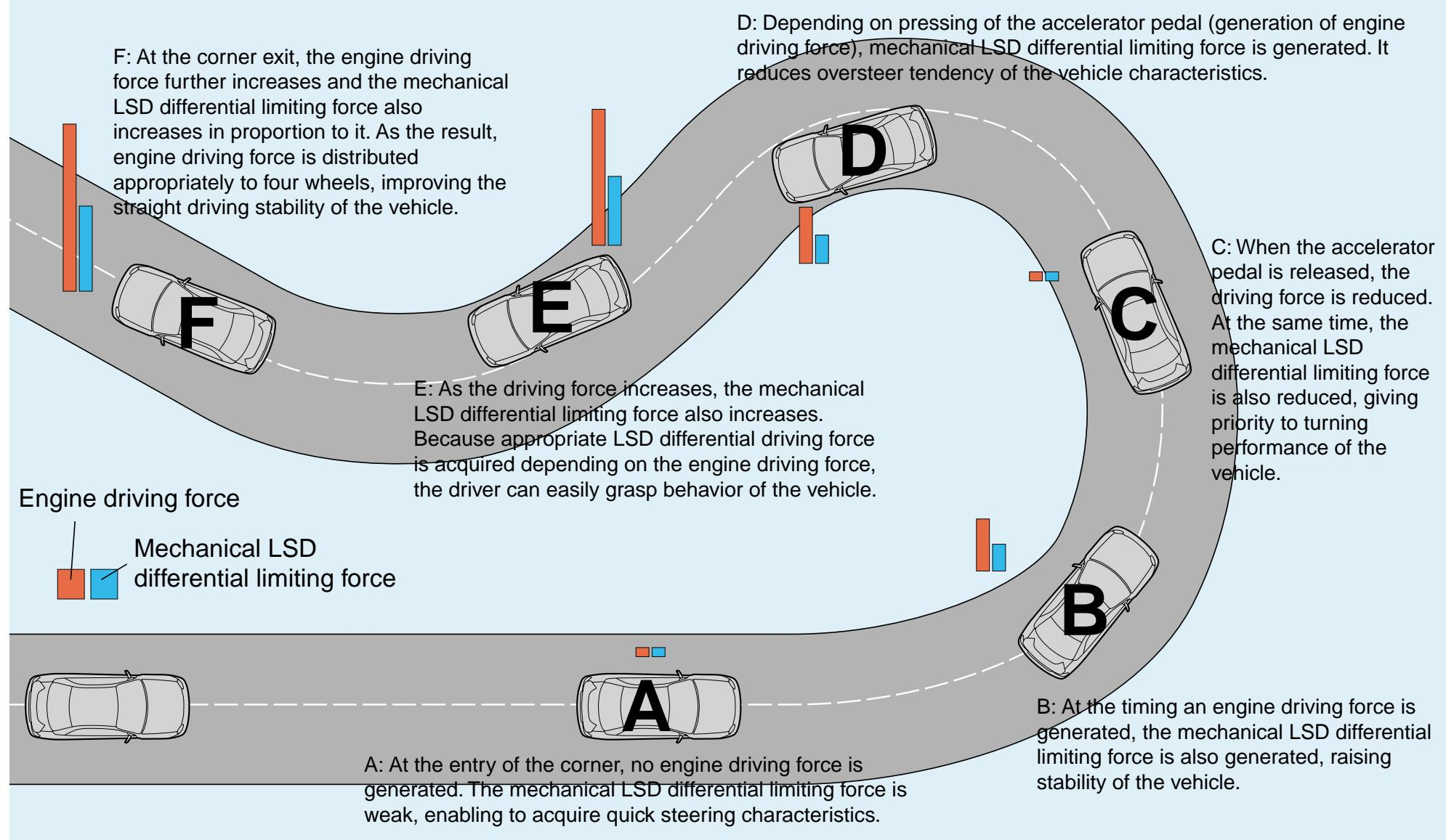
As described above, new DCCD system employing the mechanical LSD mechanism allows the timings of generating LSD differential limiting force to precisely follow the acceleration/deceleration timings of the vehicle. In addition, the differential limiting force is proportional to the engine driving force. Thus, the driver can easily grasp behavior of the vehicle and control the vehicle more freely.
